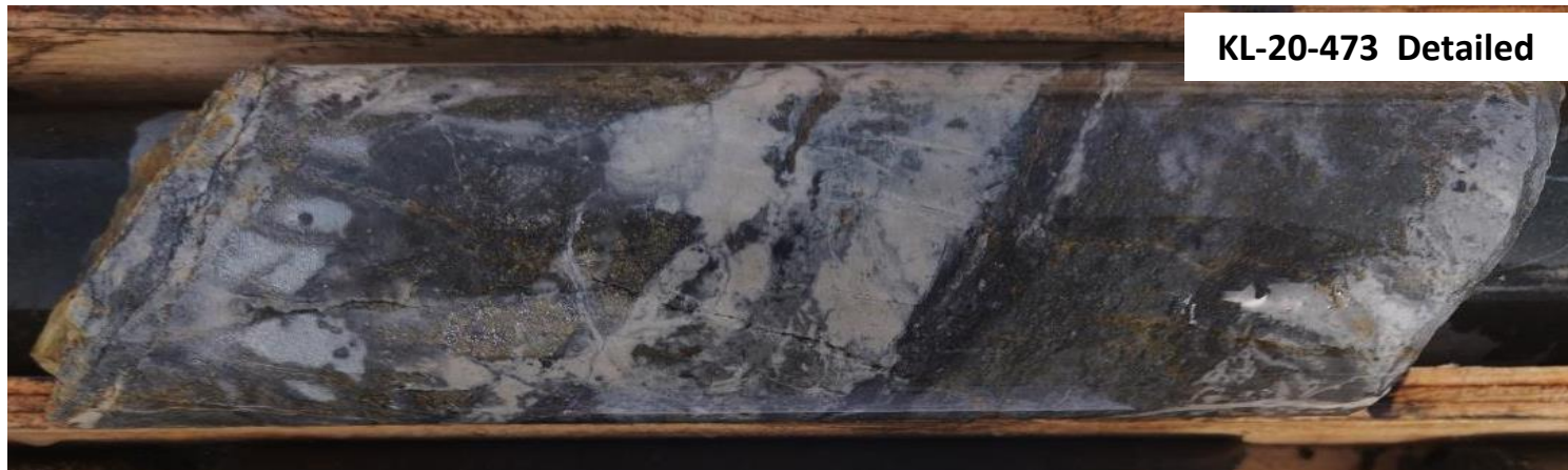
KL-20-473 115.80 m - Interval returned 6.17 g/t gold, 229.76 g/t silver, 0.84% lead and 0.57% zinc over 1.37 m
