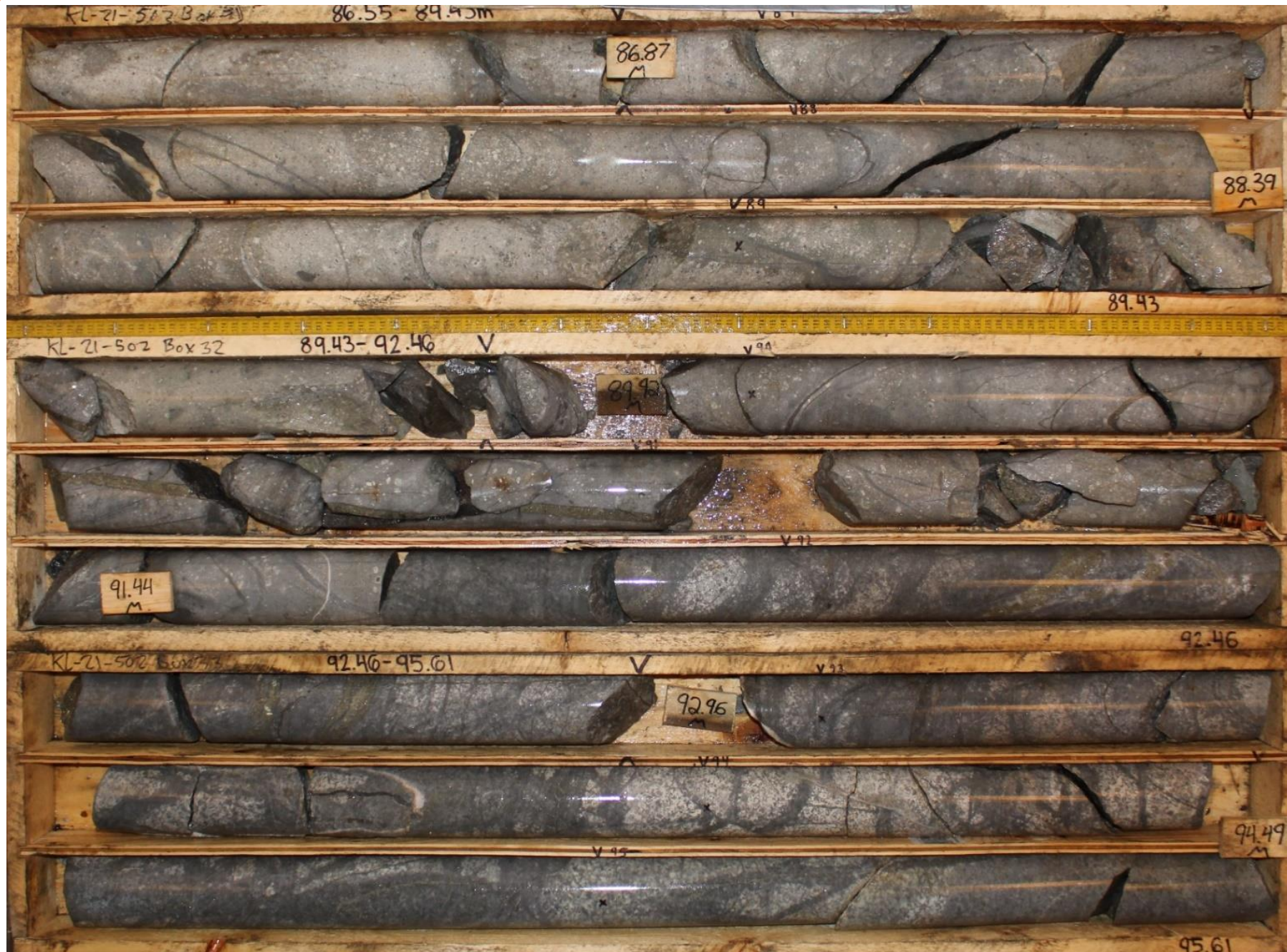
KI-21-502 – Casino Suite porphyry (upper) and Argillic altered Whitehorse Suite granodiorite (lower) hosting quartz-sulphide veins (py+cpy+minor moly)
