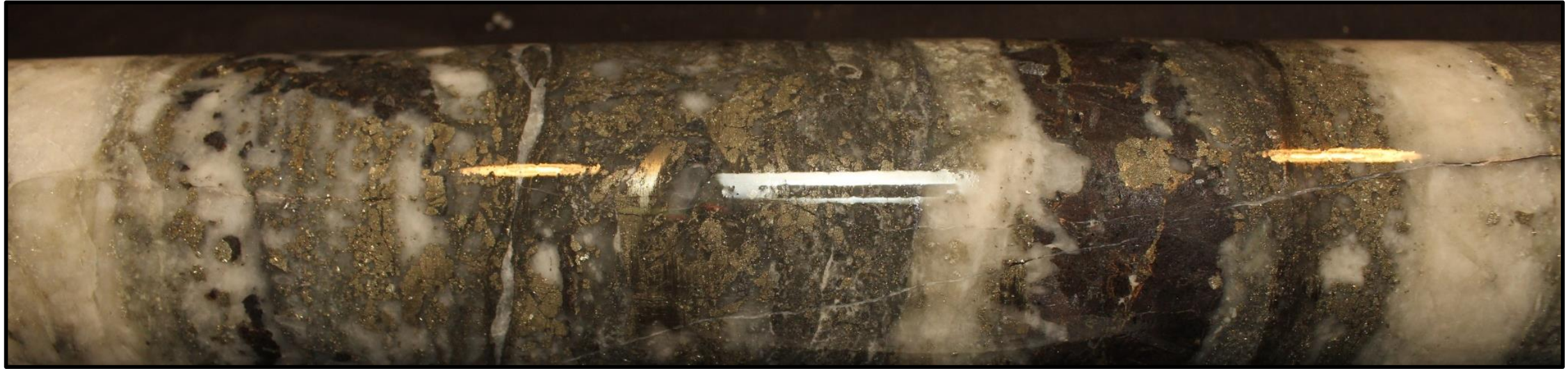
KL-15-262 144.87 m - Interval returned 31.60 g/t gold, 100 g/t silver, 0.17% lead and 6.67% zinc over 0.31 m
