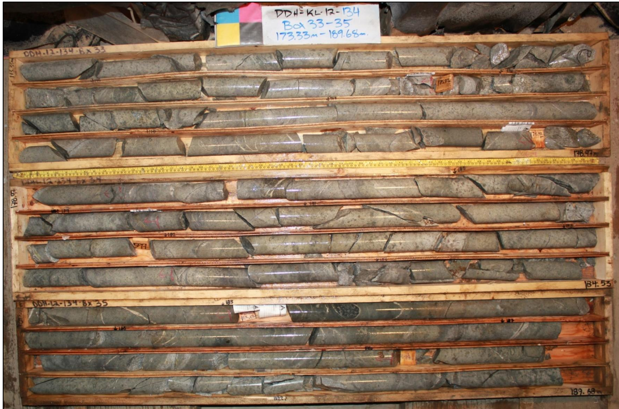
KL-12-134 Sampled interval returned 0.15% copper, 0.01% molybdenum, 0.14 g/t gold and 2.7 g/t silver over 95.15m
