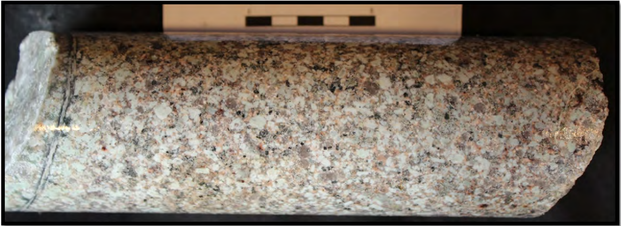
Plate 13: Moderate potassic alteration with secondary biotite.
