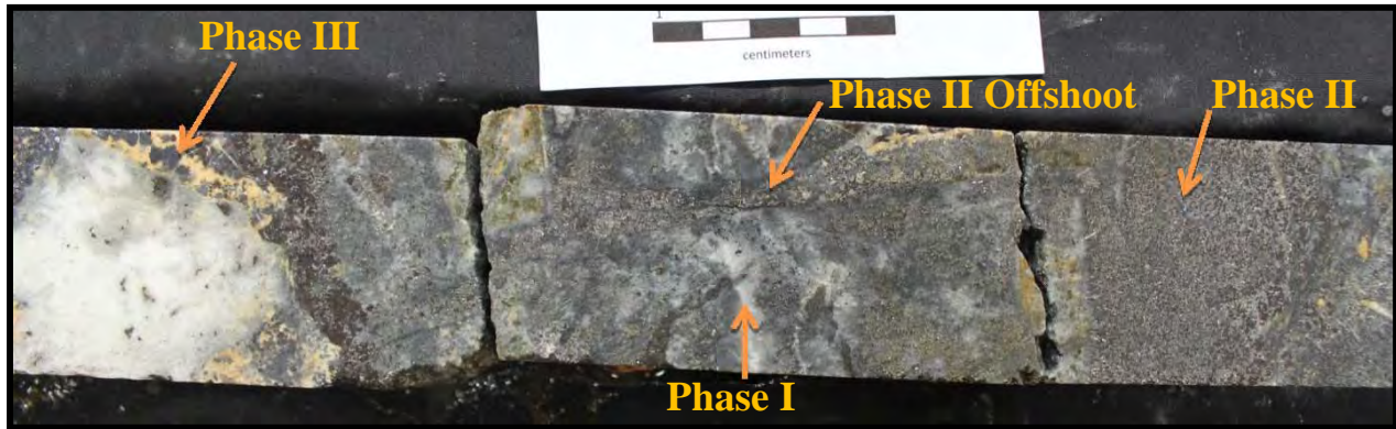
Plate 4: Western Klaza Zone drill core highlighting relationship between Phases I through III.
