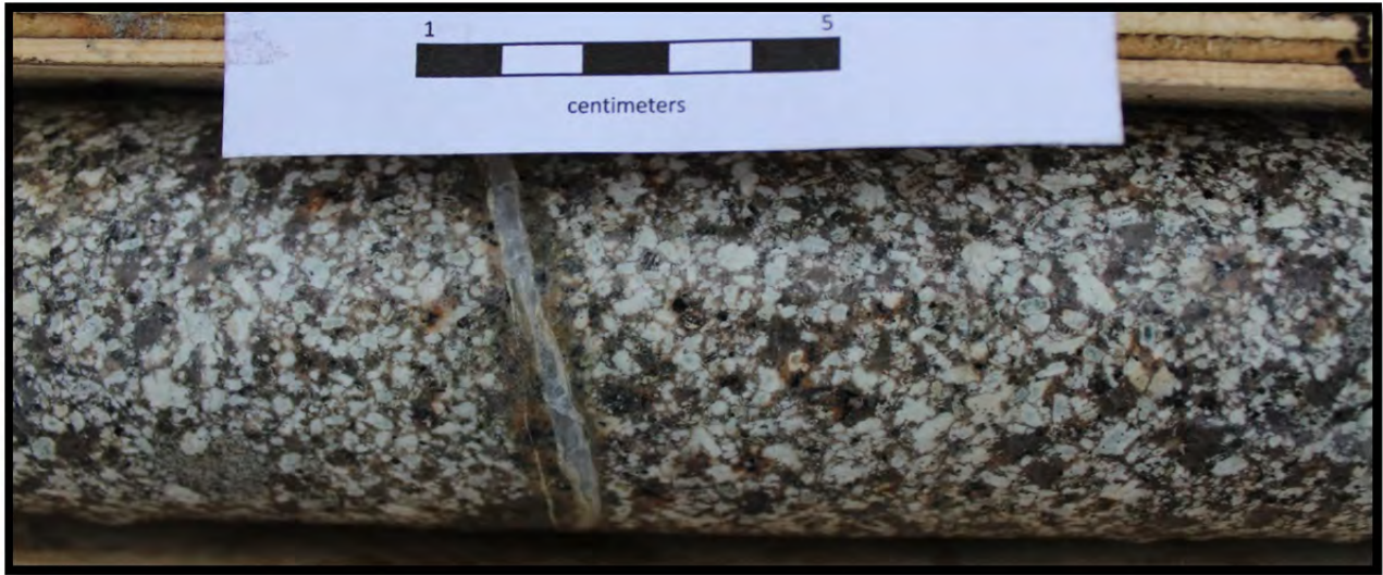
Plate 9: Weak kaolinitic alteration.
