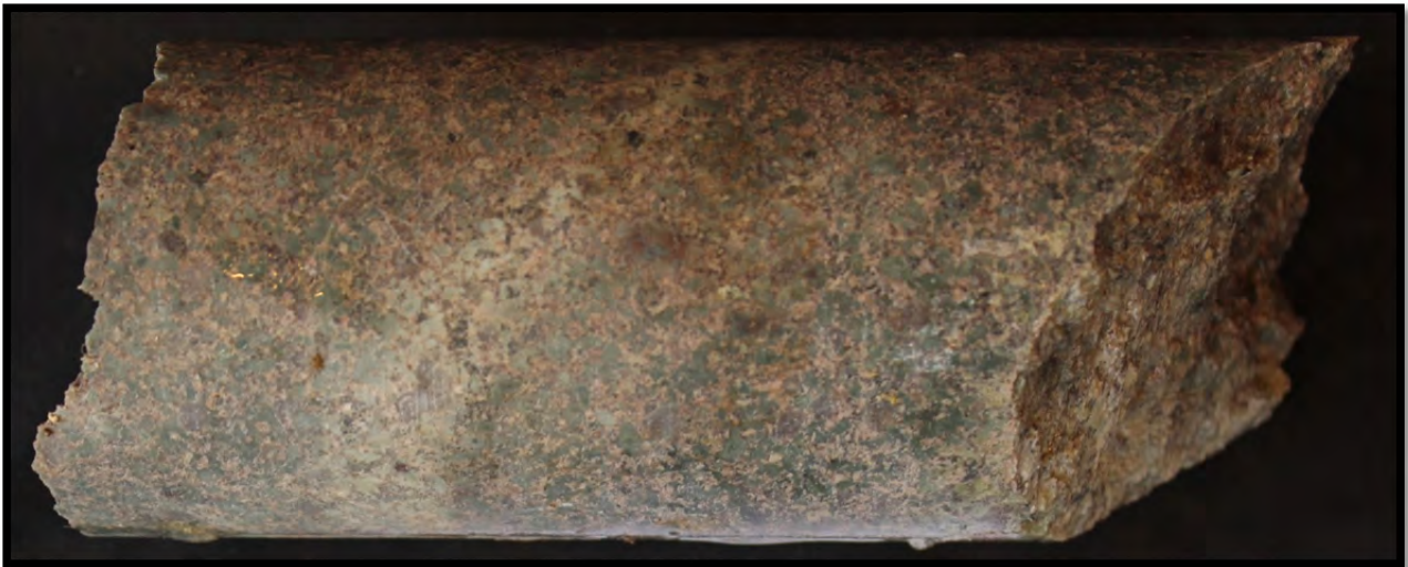
Plate 7: Strong propylitic alteration with weak potassic overprinting.
