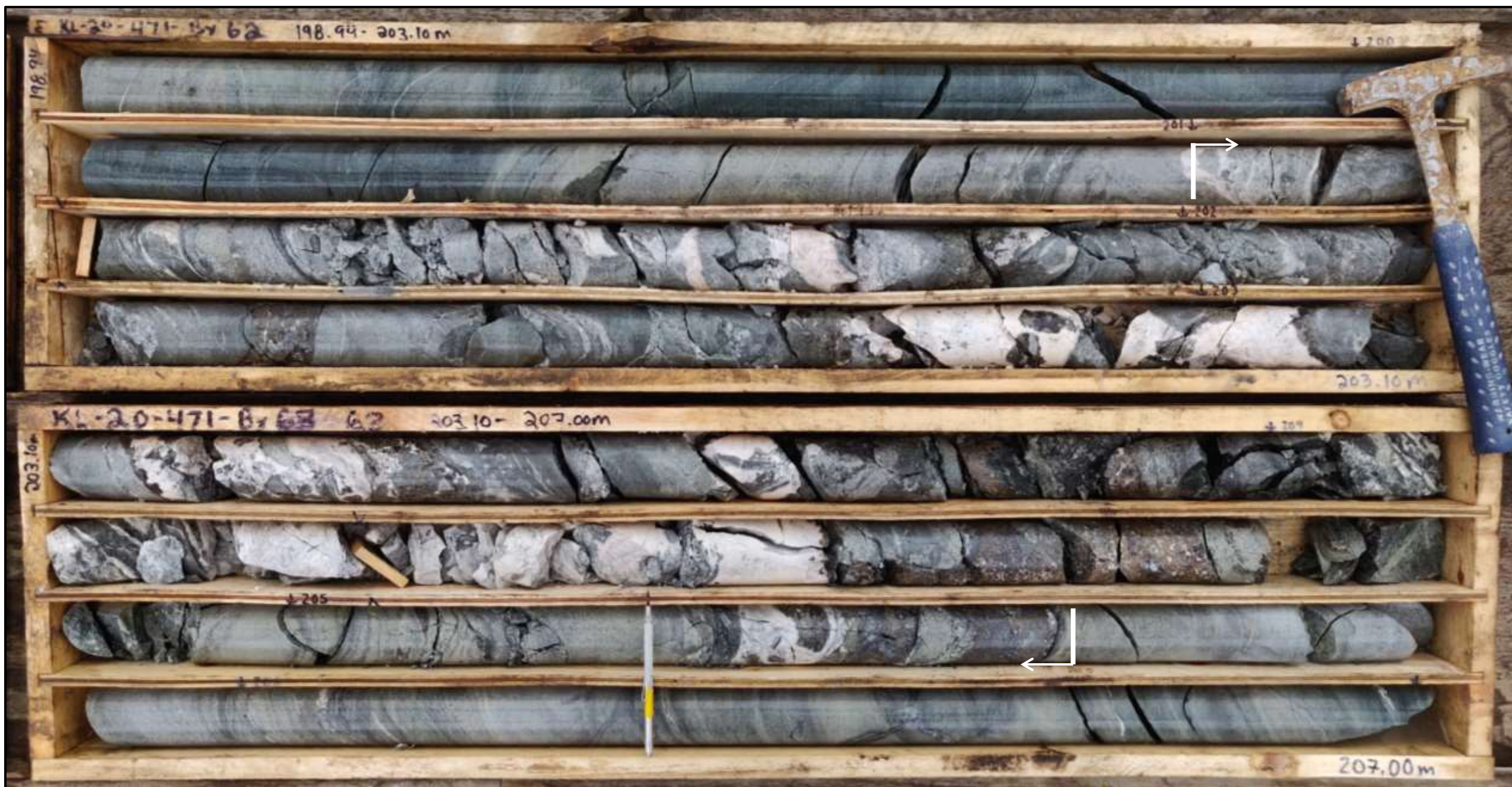
KL-20-471 201 m - Interval returned 2.05 g/t gold, 129.00 g/t silver, 2.29% lead and 4.67% zinc over 5.65 m
