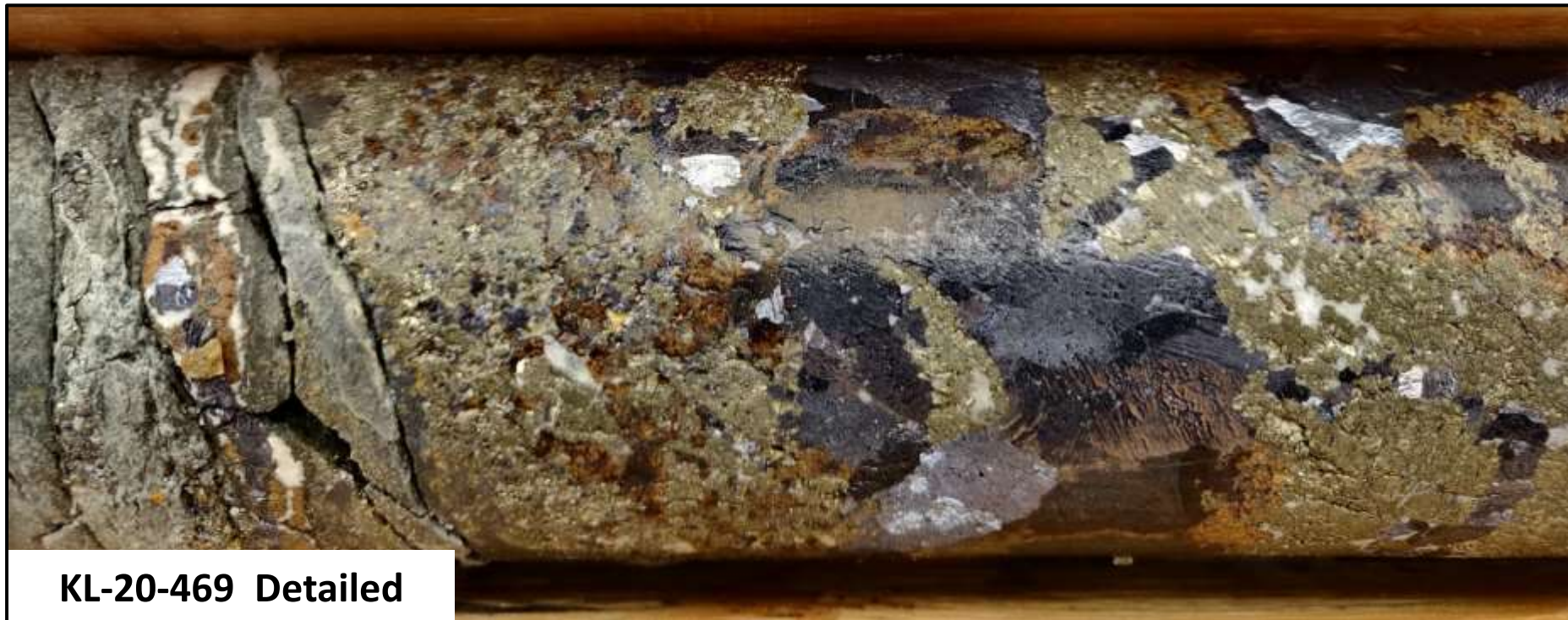
KL-20-469 82.63 m - Interval returned 2.10 g/t gold, 656.60 g/t silver, 12.98% lead and 6.17% zinc over 1.00 m
